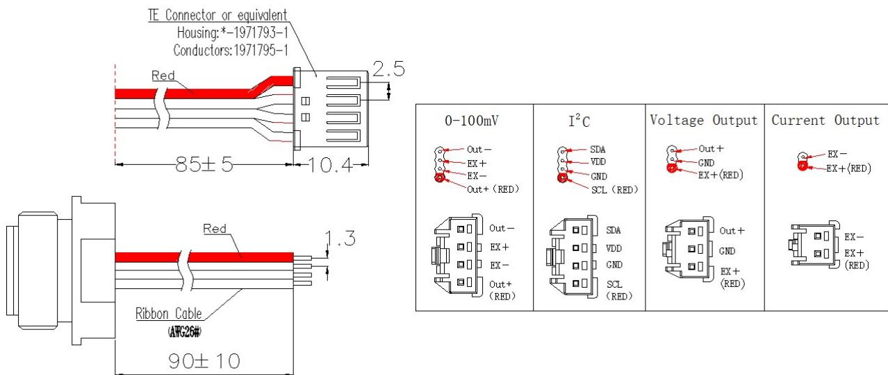
**Recommended mounting dimensions (unit:mm)**
