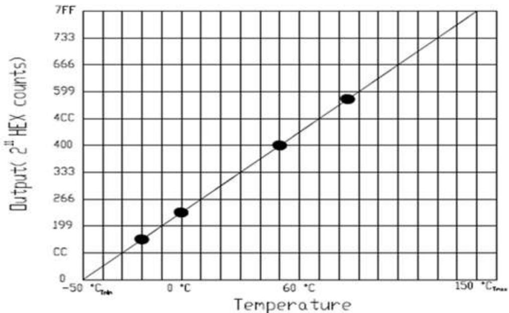
$$\text{Output (Decimal Counts)} = \frac{(\text{Output } ^\circ\text{C} - (-50^\circ\text{C})_{T_{\text{min}}}) * 2047}{(150^\circ\text{C}_{T_{\text{max}}} - (-50^\circ\text{C})_{T_{\text{min}}})}$$
