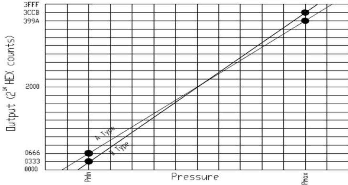
$$\text{A Type: Output (Decimal counts)} = \frac{80\% * 16383}{P_{\text{max}} - P_{\text{min}}} * (\text{Pressure}_{\text{applied}} - P_{\text{min}}) + 10\% * 16383$$
